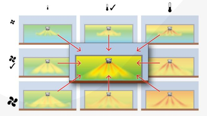
Automatically adjusting heat output and fan speed means there is always sufficient heat to warm the inducted air and there is always sufficient air speed to ensure it reaches the floor.
